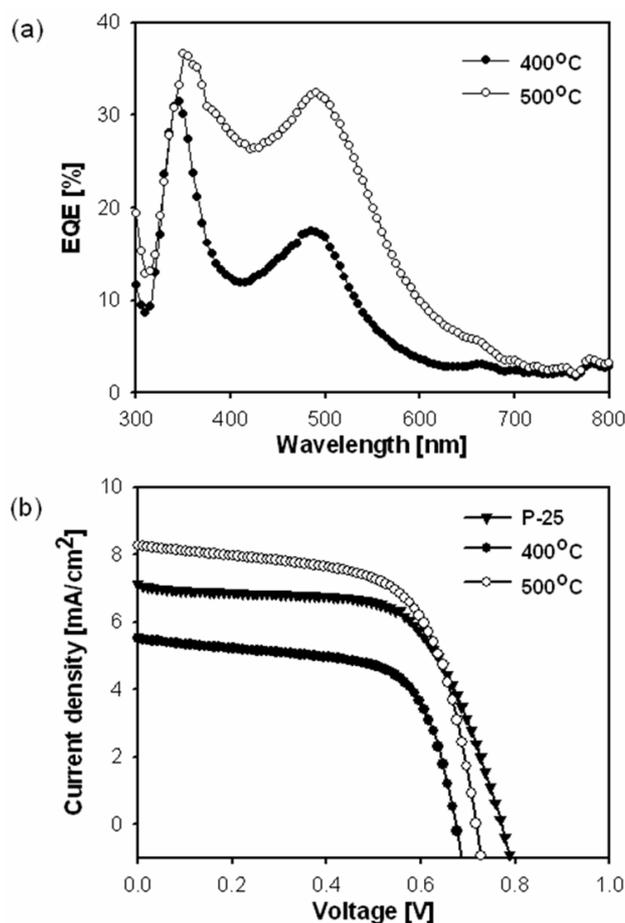
**Figure 3.** Characteristics of DSSCs. IPCE spectra (a) and photocurrent density–voltages curves (b) of TiO<sub>2</sub> nanoribbons calcined at 400 °C (filled circles) and 500 °C (unfilled circles), respectively. The device performance of commercial TiO<sub>2</sub> nanoparticle (Degussa, P-25)-based DSSCs is plotted for comparison.
