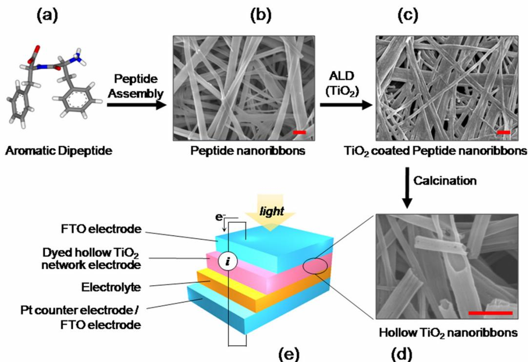
**Figure 1.** Schematically illustrated process for highly entangled hollow TiO<sub>2</sub> nanoribbons and DSSCs. (a) Molecular structure of diphenylalanine. (b) SEM image of 3D xerogel consisting of peptide nanoribbons. SEM images of the entangled TiO<sub>2</sub> nanoribbons (c) before and (d) after the calcination of the peptide template. (e) A cross section of DSSCs made from peptide-templating hollow TiO<sub>2</sub> nanoribbons. Scale bars: 1  $\mu\text{m}$ .
