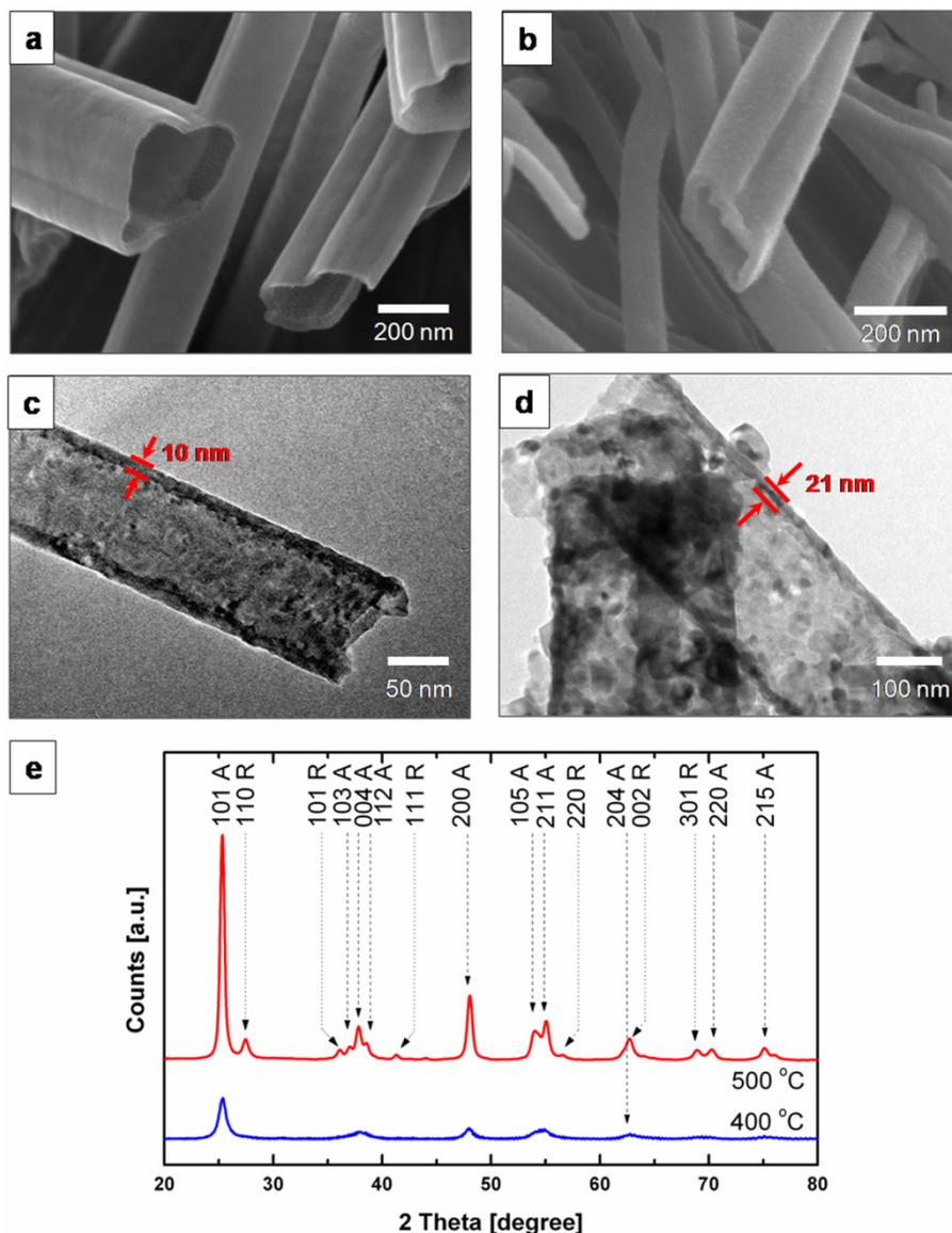
**Figure 2.** SEM and TEM images of hollow TiO<sub>2</sub> nanoribbons obtained by calcining at 400 °C ((a) and (c)) and 500 °C ((b) and (d)). (e) XRD patterns of hollow nanoribbons obtained by calcining at 400 °C and 500 °C, respectively.
