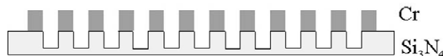
Fig. 1. Schematic cross-section of a diffraction grating. Typically the Cr layer was 25 nm-thick and the etch depth into \text{Si}_3\text{N}_4 membrane was 40 nm.
